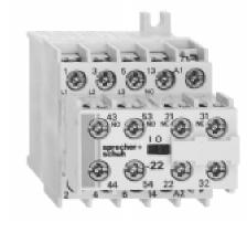
Also, due to its sideways switching movement, the basic contactor has the same low profile whether an AC or DC operating magnet is used. This permits the use of enclosures with shallow mounting depths. Once the CA4 is installed, all auxiliary contact blocks can be snapped-on or removed without changing any existing power wiring. Other accessories include a snap-on RC Link (surge suppressor), mechanical interlocks and space saving adaptors for connecting auxiliary components.
