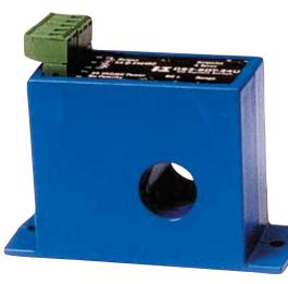
**DS3 Series** Current Operated Switches combine a Hall effect sensor, signal conditioner and a limit alarm into a single package. The DS3 Series offers three jumper-selected current input ranges and frequency response from DC to 400Hz. Available in a solid-core case with choice of relay or a universal solid-state output.
