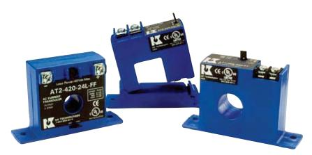
AT Series Current Transducers combine a current transformer and signal conditioner into a single package. The AT Series has jumper selected current input ranges and industry standard 4–20mA, 0–5VDC or 0–10VDC outputs. The AT Series is designed for application on 'linear' or sinusoidal AC loads. Available in a split-core case or two types of solid-core cases.
