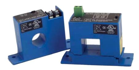
**ATR Series** Current Transducers combine a current transformer and a True RMS signal conditioner into a single package. The ATR Series provides True RMS output on distorted waveforms found on VFD or SCR outputs, and on linear loads in "noisy" power environments. Available in a solidor split-core case.
