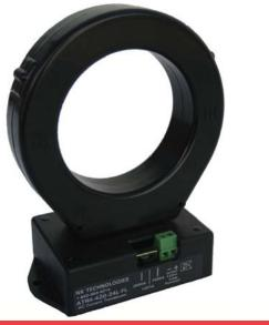
**ATP/ATPR 3 & 4 Series** Powered High-Current Transducers are largeformat solid-core transducers designed for high current applications from 200A to 2000A. Powered by 120VAC or 24VAC/VDC, these products take advantage of available power supplies and eliminate the need for costly control power transformers. Options include average responding and True RMS versions, 0–5/10VDC or 4–20mA analog outputs and switch-selectable input ranges.
