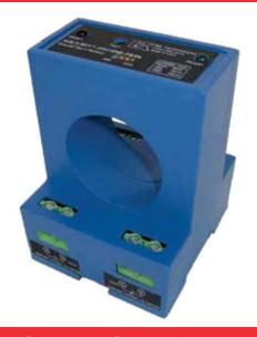
AGL Series, new from NK Technologies, is a large aperture ground fault sensor that offers one of the largest aperture diameters in the industry while maintaining a compact overall profile. Intended for sensing earth leakage in applications up to 600A, the AGL Series offers a choice of N.O. or N.C. latching relays or an SPDT Form C relay with auto-reset. Enclosure features integral DIN-rail mounting as standard and optional noise immunity coatings for applications in harsh EMI/RFI environments.
