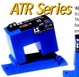
ATR Series from NK Technologies combine a current transformer and a True RMS signal conditioner into a single package. The ATR Series provides True RMS output on distorted waveforms found on VFD or SCR outputs and on linear loads in "noisy" power environments. Available in a solid or split core case.
