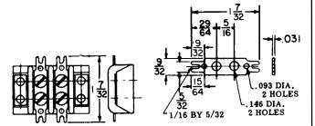
This is an assembly of the 37TB Class Terminal Board and a two-sided terminal lug (TBLD). Available in lengths from 2 terminal (37TBLD-2) through 31 terminals (37TBLD-31). Lugs are brass per QQ-B-613 and are tin plated.
