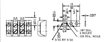
This is an assembly of the 39TB Class Terminal Board and a one-sided terminal lug (TBLS). Available in lengths from 2 terminal (39TBLS-2) through 18 terminals (39TBLS-18). Lugs are brass per QQ-B-613 and are tin plated.
