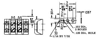
This is an assembly of the 38TB Class Terminal Board and a one-sided terminal lug (TBLS). Available in lengths from 2 terminals (38TBLS-2) through 23 terminals (38TBLS-23). Lugs are brass per QQ-B-613 and are tin plated.
