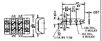
This is an assembly of the 38TB Class Terminal Board and a two-sided terminal lug (TBLD). Available in lengths from 2 termianl (38TBLD-2) through 23 terminals (38TBLD-23). Lugs are brass per QQ-B-613 and are tin plated.
