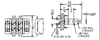
This is an assembly of the 39TB Class Terminal Board and a two-sided terminal lug (TBLD). Available inlengths from 2 terminal (39TBLD-2) through 18 terminals (39TBLD-18). Lugs are brass per QQ-B-613 and are tin plated.
