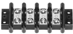
Base, General Purpose Phenolic, 150° C JJ (GDI-30F) Material is Available Open Back Design Screws, #12-32 Binder Head, Phil-Slot Terminals, Plated Brass 1-8 Poles 14/16" Centers Wire Range with Wire Binding Screw #4 - #12 Awg - 70 Amps The Suitability of These Devices for Greater Currents Shall Be Determined in the End-Use Application. UL Recognized File No. E47811 CSA Certified File No. LR19766 CE
