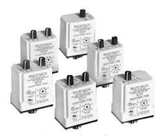
Voltage Monitor Relays monitor either AC single phase (50-60Hz) or DC voltages to protect equipment against voltage fault conditions. No separate supply (input) voltage is required on any Macromatic Voltage Monitor Relays. All versions are available in a compact plug-in case utilizing an 8 pin octal socket.
