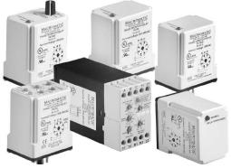
Phase Monitor Relays provide protection against premature equipment failure caused by voltage faults on 3 Phase systems. All Macromatic Phase Monitor Relays are designed to be compatible with most Wye or Delta systems with no connection to Neutral required. Phase Monitor Relays protect against single phasing regardless of any regenerative voltages.
