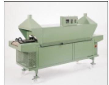
Large high performance industrial tunnel ovens often utilized for automotive hose and pipe applications. Features include the following:
