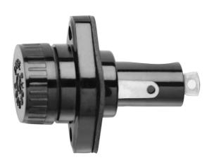
Catalog Symbol: HPC-D Waterproof Panel-Mount Ampere Rating: 30 Amperes Voltage Rating: 600 Volts AC Agency Approvals: U.L. Recognized, Guide IZLT2, File E14853 U.L. Flammability Rating: 94 VO Temperature Rating (RTI): 150°C
