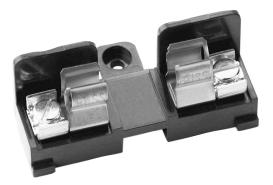
Catalog Symbol: 3743 Add-On Fuseblocks Ampere Rating: 30 Amperes Voltage Rating: 600 Volts AC Temperature Rating (RTI): 150°C Agency Approvals: U.L. Recognized, Guide IZLT2, File E14853
