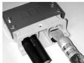
Figure 1: Contact insertion orientation
