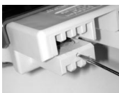
Figure 2: Screwdriver insertion for contact removal
