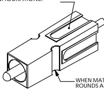
WHEN MATED SIDE TO SIDE, HALF-ROUNDS ALIGN TO FORM A SLOT FOR ROLL PIN INSERTION, WHICH PROTECTS AGAINST ACCIDENTAL DISLODGING OF MATED HOUSINGS.
