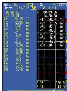
Standard Measurement Screen (Measured values appear numerically at the left, and plotted as a graph at the right together with the measured values at the cursors.)
